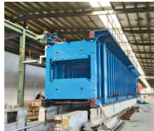
Re-assembly of ContiRoll® press frames
