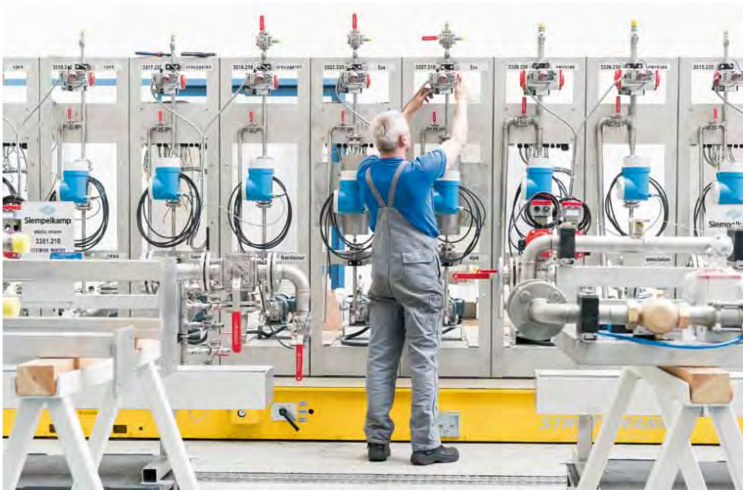
Assembly of glue kitchen with modular design
