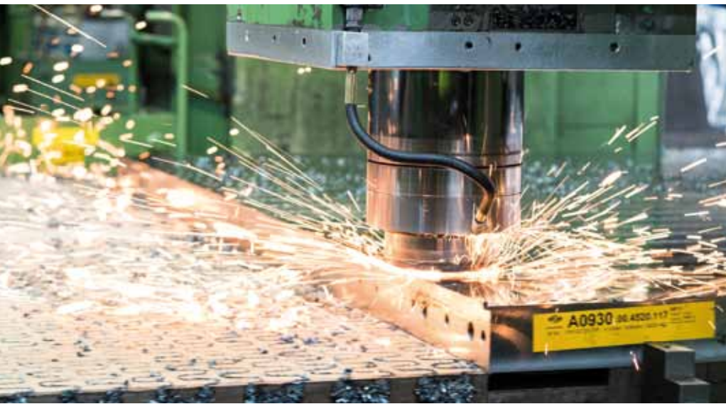
Milling of a hot platen
